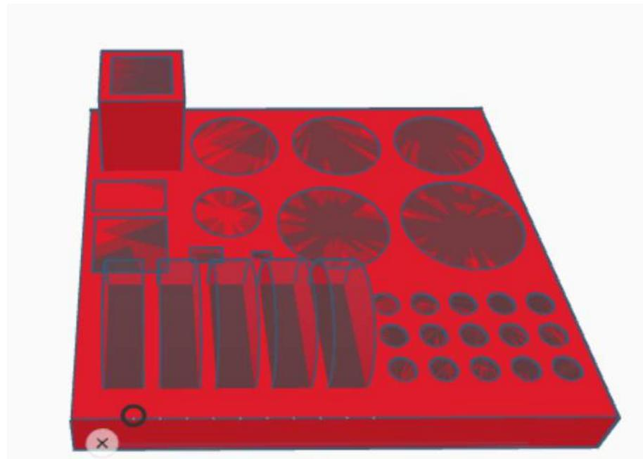
In the finished design, everything that appears as a dark gray shape is a “hollow.” When combined with the solid red base, these hollows remove material, which is how I was able to create snug cradles for items like the Pan Pastels and glue bottles. It’s a simple concept, but incredibly powerful when designing custom storage. Here you can see the completed Tinkercad file before printing.
