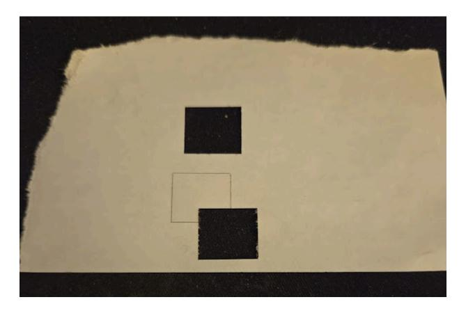
I did it! Yes!!! What's noticeably absent from this picture? Char marks along the edges of the path of the laser. The air assist is doing its job in perfect form to prevent the charring of the delicate paper. Suddenly my fears have been washed away, and the only hing that remains is possibility!
