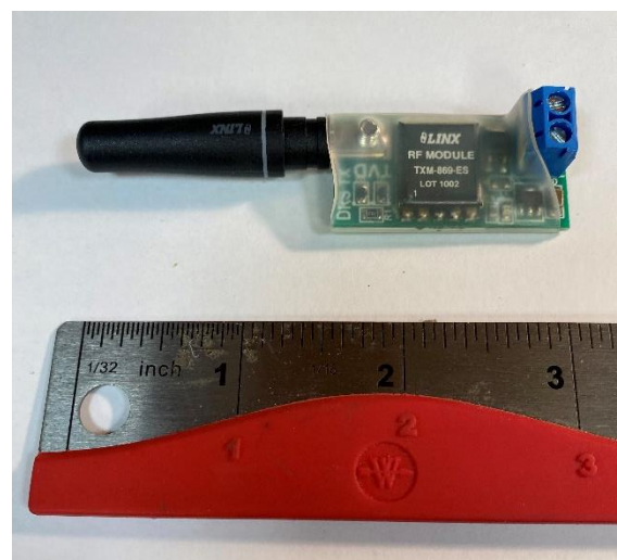
This Linx RF module transmits the DCC commands to the receiver (picture on left) mounted in the locomotive tender.
