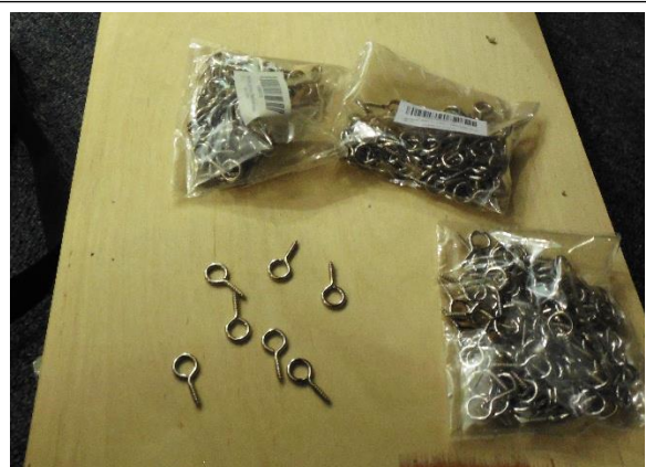
Pic 8: I'm using screw eyes to support wire runs under the layout.
