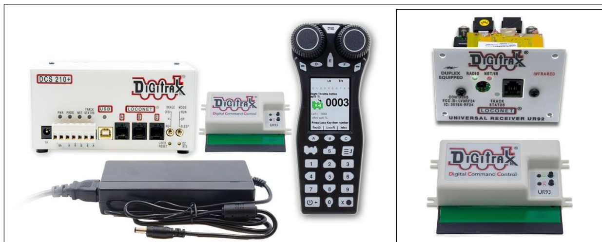
Pic 3: Upgrading to the Evolution Duplex set includes the items shown on the left. This also replaces the older UR92 Receiver (inset top) with the newer UR93 (inset bottom).
