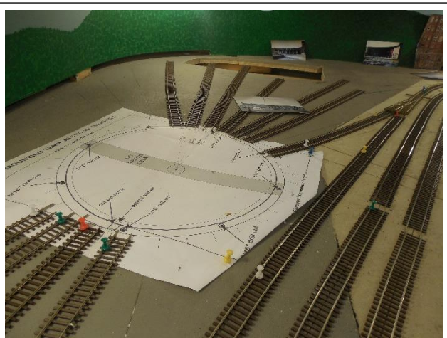
Picture 8 – Template and rough-in layout of tracks leading into and from the 90' turntable. The roundhouse will be scratchbuilt.
