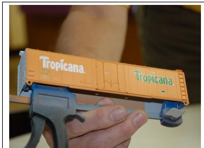
Notice how the flat coat on the left makes the decal film disappear compared to the right side.
