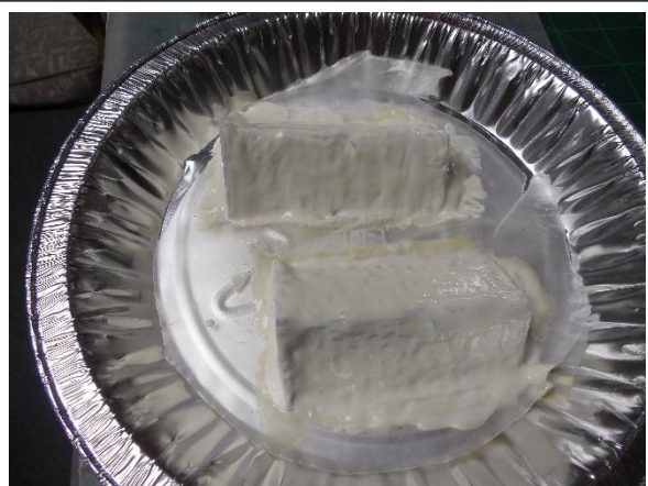
Figure 6 – Pouring Hydrocal into molds.
