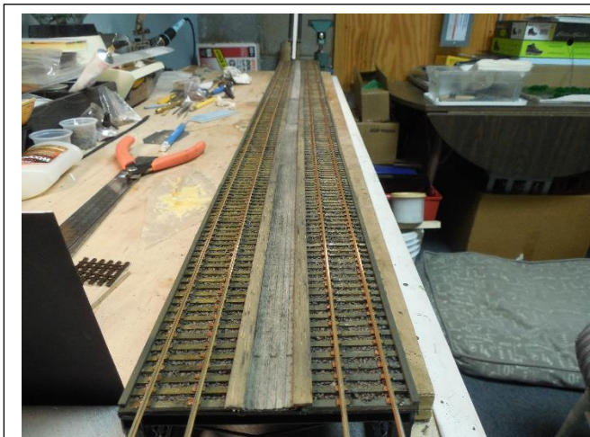
Fig 20 – Northeastern scale lumber was used for the walkway on the bridge deck.
