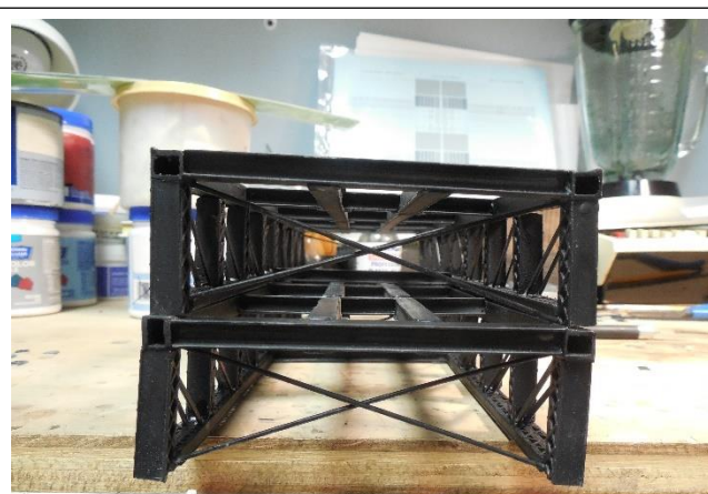
Fig 7 – An end view of the bridge sections show some of the internal bracing installed.
