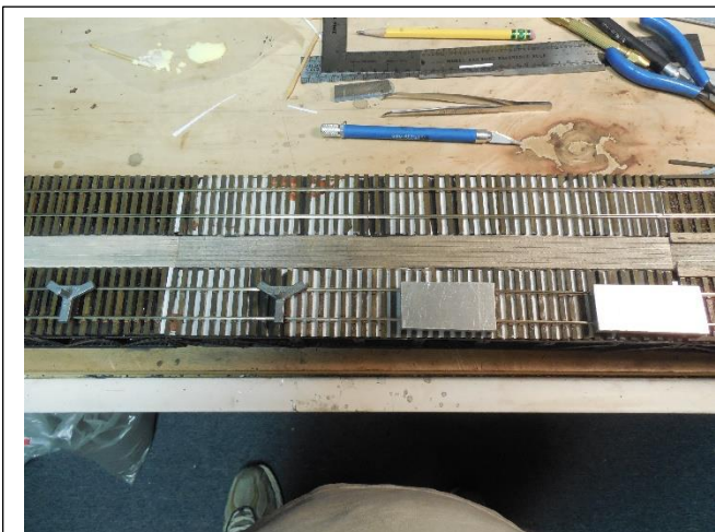
Fig 14 – Hand laying code 83 rail into place onto the tie plates.
