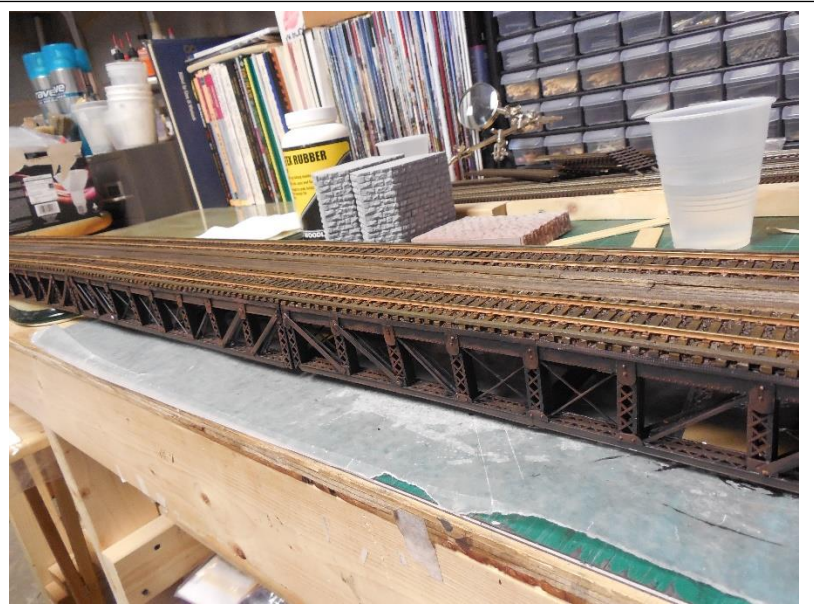
Fig 23 – Track, walkway and bridge sides are weathered and all four bridge sections are joined together.
