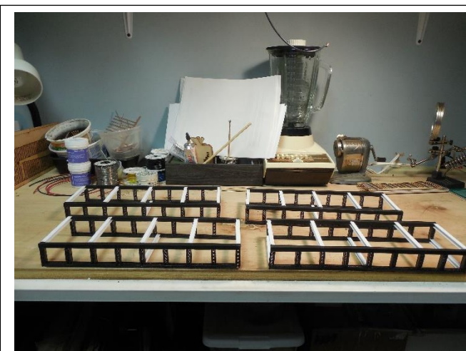
Fig 4 – The basic bridge sections were built using styrene girders and shapes.
