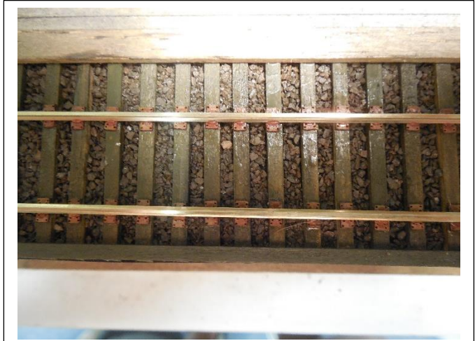
Fig 17 – The hand laid rail looks good against the laser cut tie plates.
