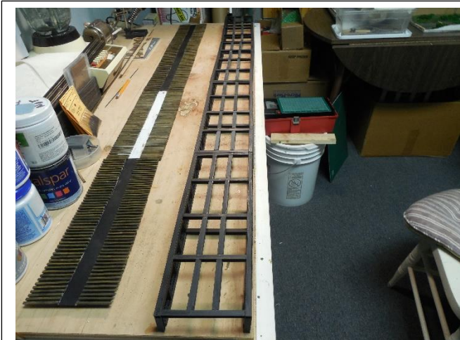
Fig 10 – Bridge ties were cut, stained and secured to the bridge deck pieces.
