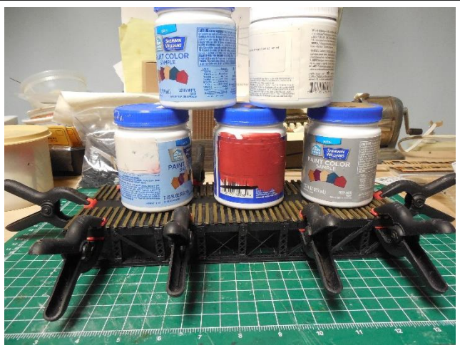
Fig 11 – Bridge ties weighted down during a glue test that showed good adhesion to a painted surface.
