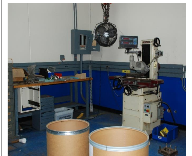
A traditional machine shop includes a horizontal milling machine and other stationary tools.
