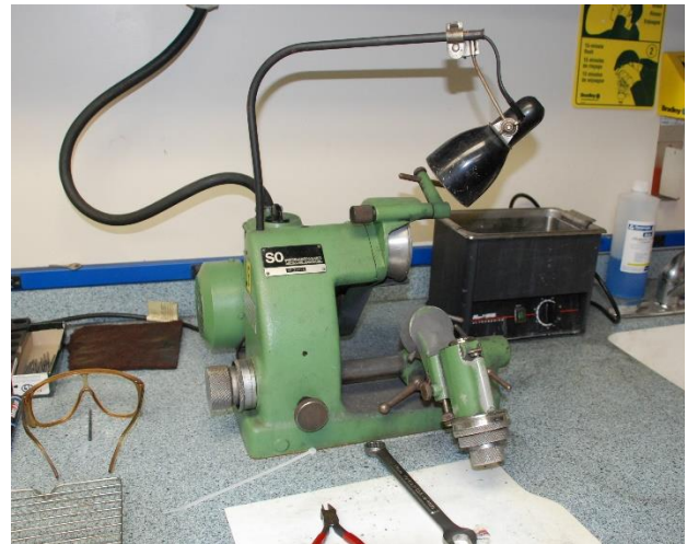
This grinding machine is used to form the cutters for the milling machine from carbide blanks.
