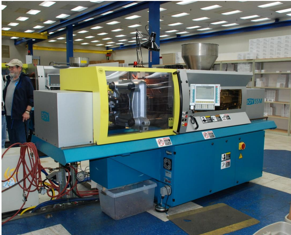
An injection molding machine happily cycles away, producing oil drums which drop into the plastic bin at the bottom after they are ejected from the mold.
