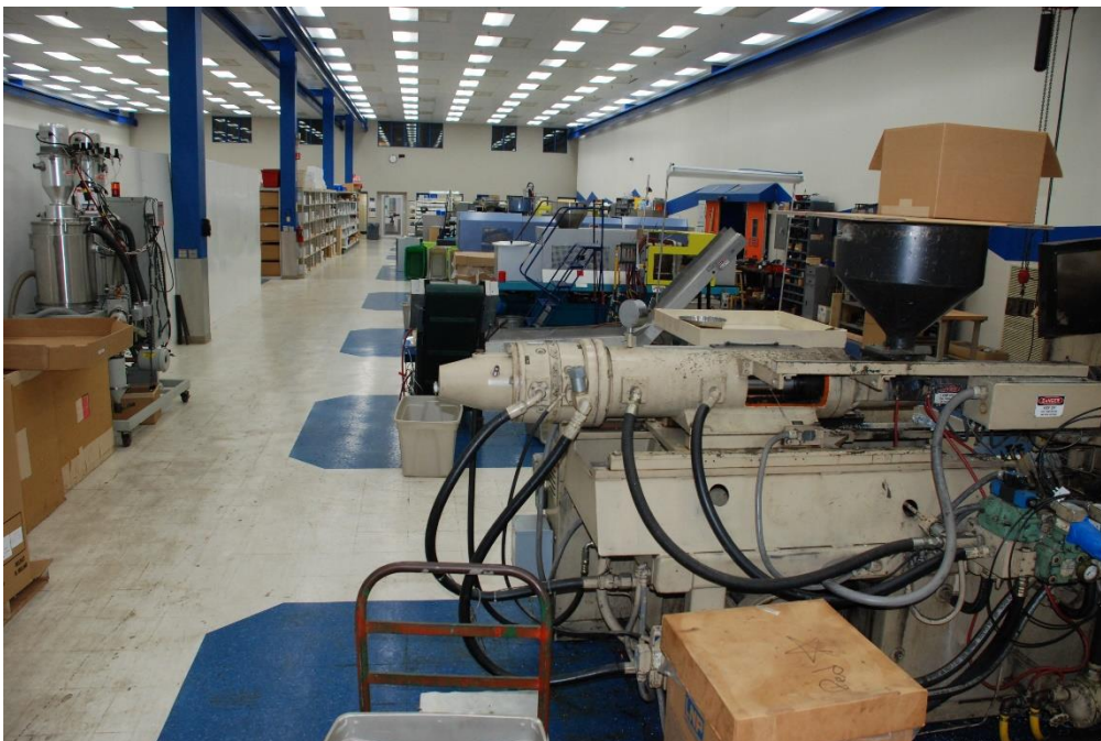
An overall view of the production machine side of the building. In the foreground is part of the largest of four injection molding machines. The large one is used for large molds (such as used for the cooling tower kit), where the molten styrene is injected at higher pressure – up to 12 tons or more.
