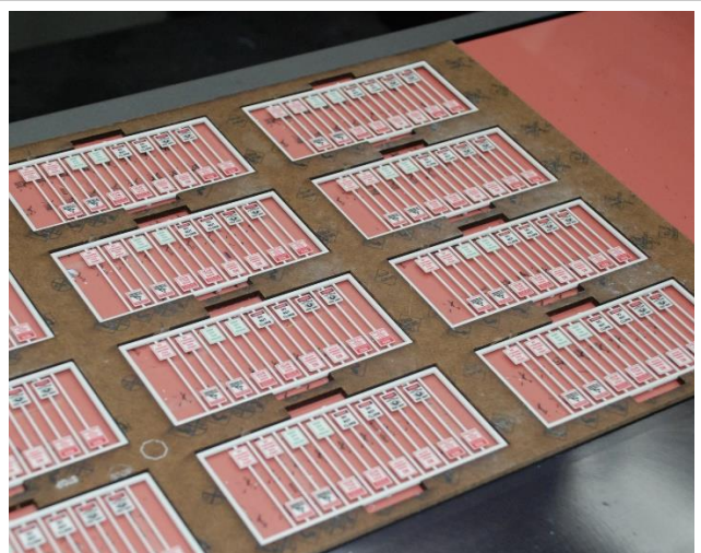
Finished signs are ready for packaging. The laser printer allows for multi-color printing in one pass.
