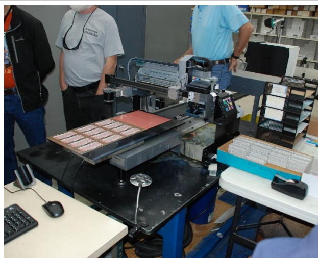
This laser printer was set up for printing signs. The blanks are stacked in the blue box to the right.
