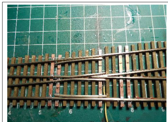
Fig 15 – Guard rails, closure rails & guards and frog soldered after checking with gauge
