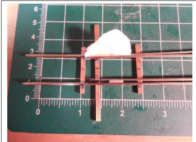
Fig 16 – Soldering point rail to throw bar
