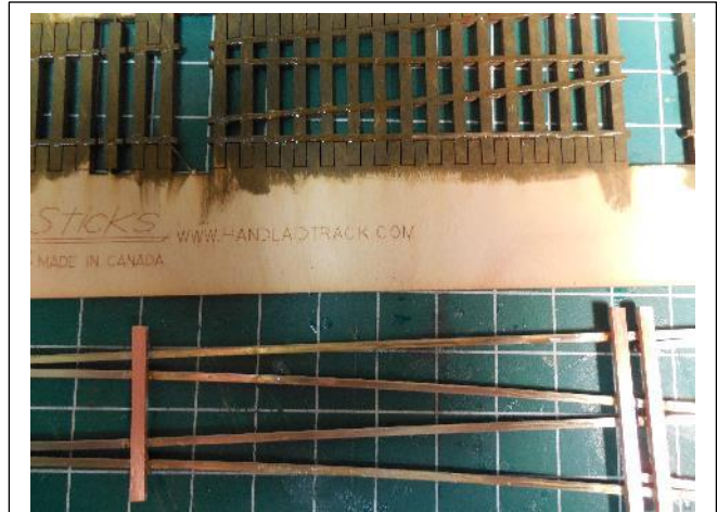
Fig 20 – Pliobond applied to ties and rail
