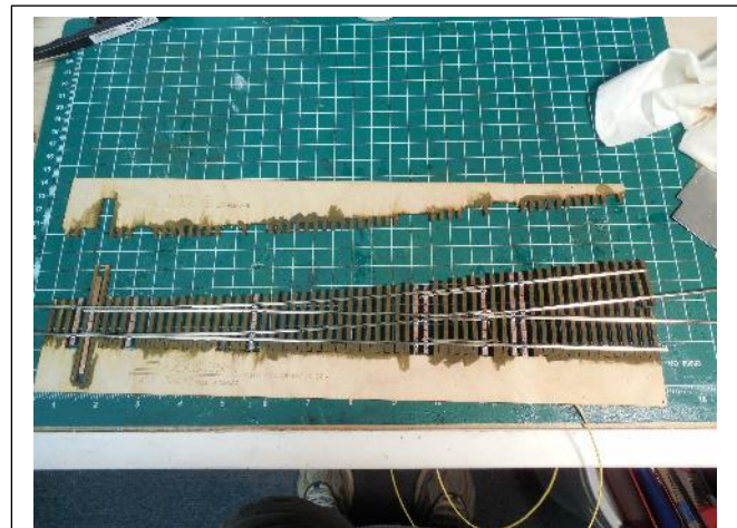
Fig 22 – Remove excess wood from laser-cut Quicksticks ties
