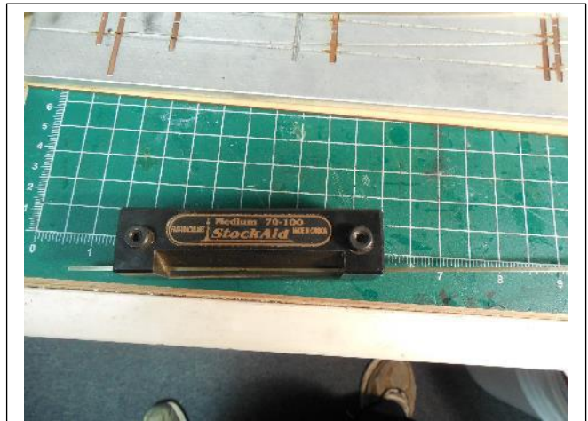
Fig 11 – Filing stock rail for where points will meet
