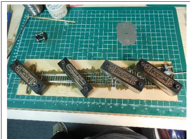
Fig 21 – Turnout on ties with weights while Pliobond sets
