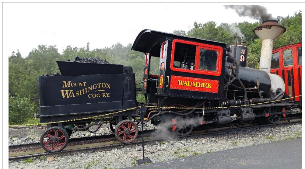
The cog steam locomotive looks like it was put on the track wrong, but it is designed this way to keep the slopesheet covered with water inside the boiler on the steep inclined track.
