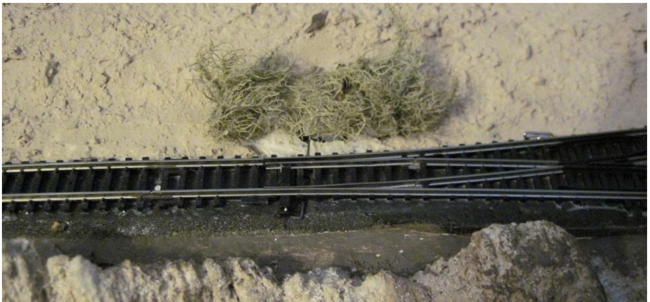
Brush used to conceal the Servo Motor
