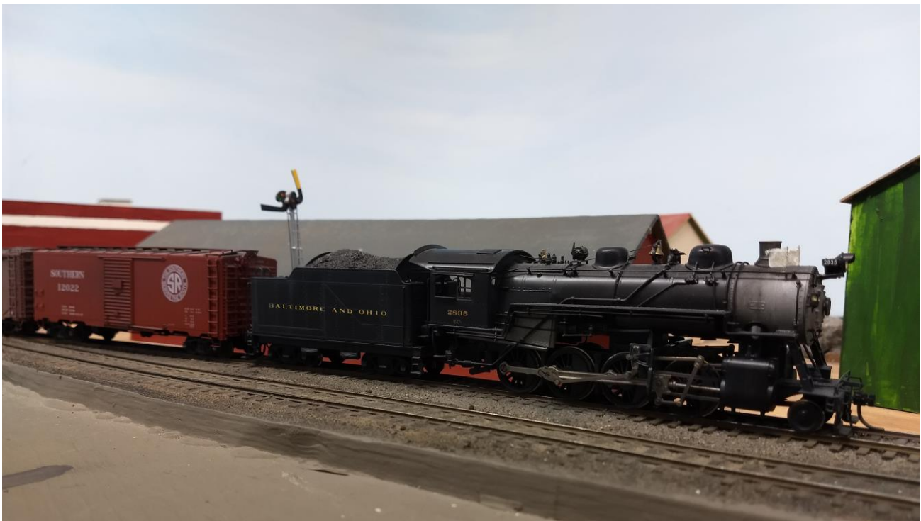
B&O class E-27b 2-8-0 #2835 shows the white flags of an extra as it pulls a cut of cars on John King's Shenandoah Subdivision. The prototype for this brass model was built by Richmond Locomotive Works in 1909, eight years after Richmond joined seven other companies to form ALCO. The small consolidation survived into the 1950s.
