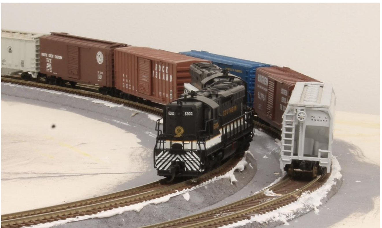
Superelevation of the main line is evident as No 165 rounds the curve in Newton.
