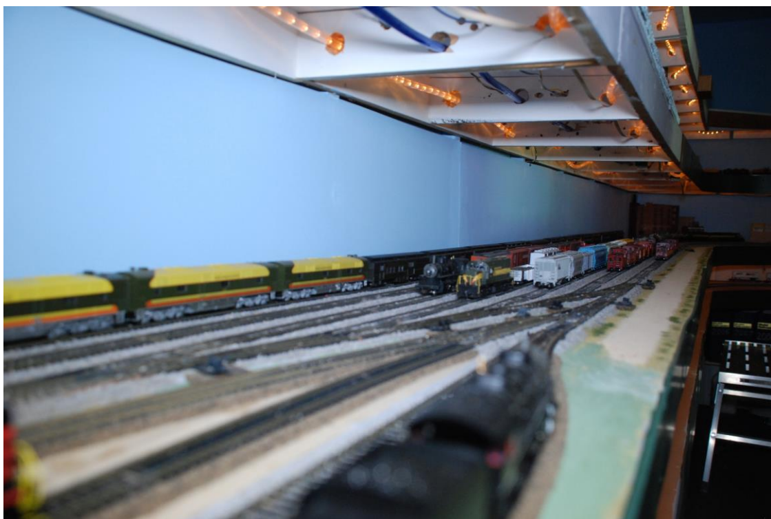
Looking in the opposite direction along the back wall shows how the multi-level benchwork provides for nice long sidings, easy access to turnouts, and a realistic feel to the layout of yard trackage. Also, notice the installation of ribbon lighting between levels
