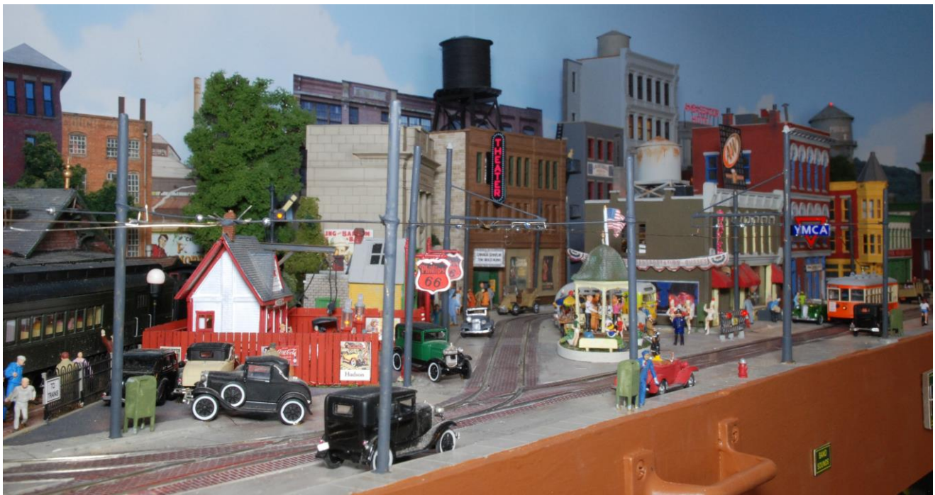
Handlaid track is imbedded in the streets. Turnouts are single point style and use cast frogs.
