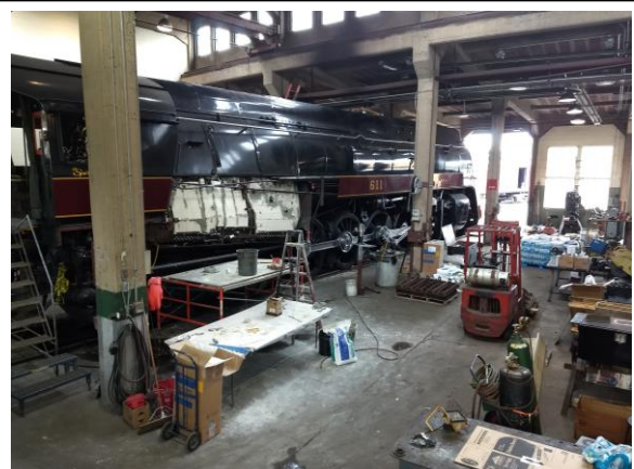
The group was treated to a view of 611 undergoing maintenance. A rare view of the insulation on the firbox with the cladding removed.
