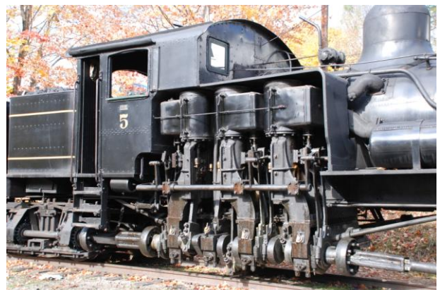
The business end of the running gear. With its vertical cylinders turning the crankshaft, power is transferred through the drive shafts to the geared trucks. Shays aren't fast, but with their gearing are able to produce exceptional torque for pulling loads up steep grades.
