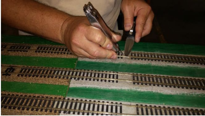
The gaps between modules are carefully closed
