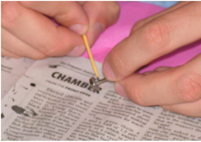
CA is applied to fill gap between axle and wheel
