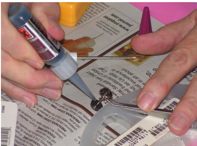
A drop of "Tire Glue" holds the resistor in position.
