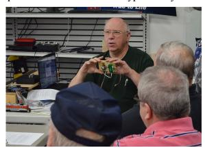
Roy shows an interface board that lets him connect a decoder to the programming track ouput of the DCC system. Board includes a motor so that the decoder can respond to commands by briefly turning motor on and drawing current from the DCC system.
