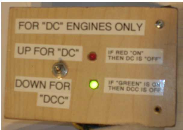
Switch is up for DC and Green LED is lit
