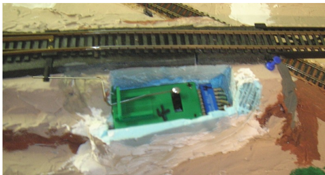
Tortoise machine in place.
