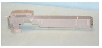
as possible. Once trimmed correctly the dynamic brake section was refitted up in the front area of the shell. Notice in the photo that the top piece of the front nose was still missing. The section was cut out by hand then adjusted with an Exacto knife and sand paper until it fit back on top of the nose and in front of the brake tubes.
