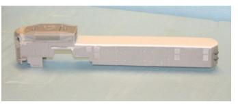
down smooth. Later two sets of vents would be added to different locations. The Dremel tool was also used to sand down the steps area around where the cab used to be. That area would need to be smooth for the next step.
